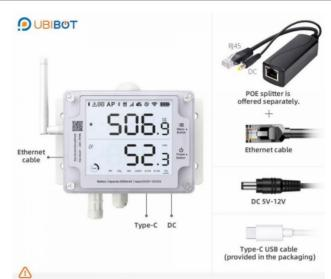
The GS1-AETH1RS device consumes a lot of power for constant performance. So We recommend you plug it to any of the external power supplies, especially the first time switch it on.
