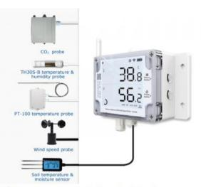
▲ Supports up to 5 probes simultaneously, 1 of each type. The TH30S-B probe is not compatible with CO₂ on some models. For details, please contact us for specific instructions.
