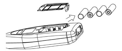
Fig 1: Opening and closing of battery cover
